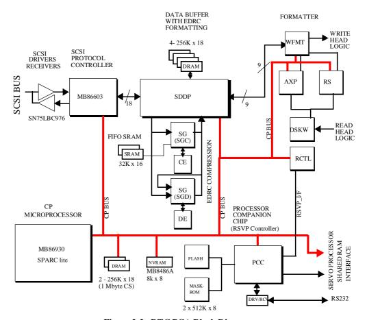
Figure 2-2. DTC PCA Block Diagram
